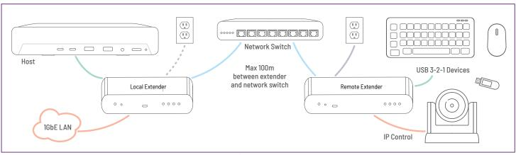
$^st$  If the host computer can deliver 15W to the Local Extender, the Local Extender power supply is not required.
